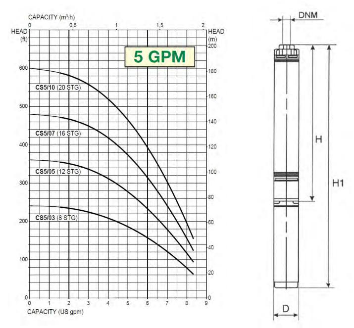
The performance curves are based on the kinematic viscosity values =  $1 \text{ mm}^2/\text{s}$  and density equivalent to  $1000 \text{ kg/m}^3$ . Curve tolerance according to ISO 9906.
